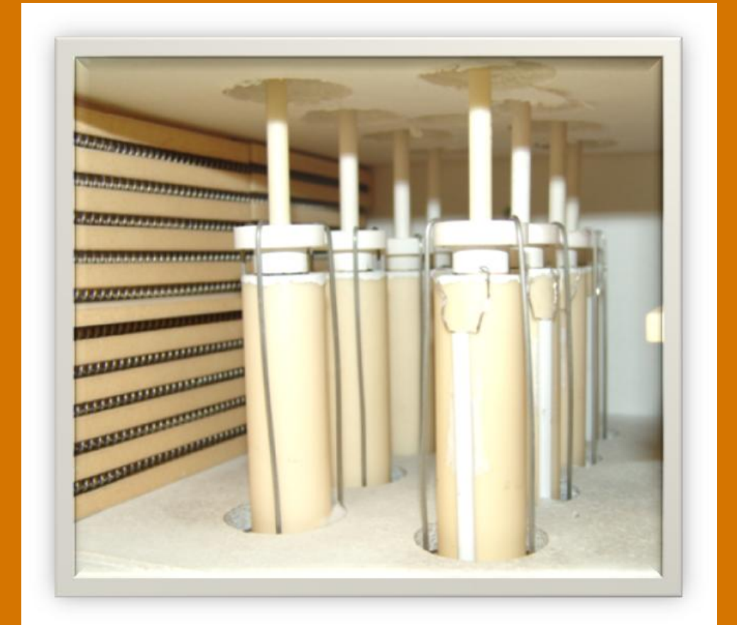
Eight button cells installed per box furnace, with individual gas flow controls
